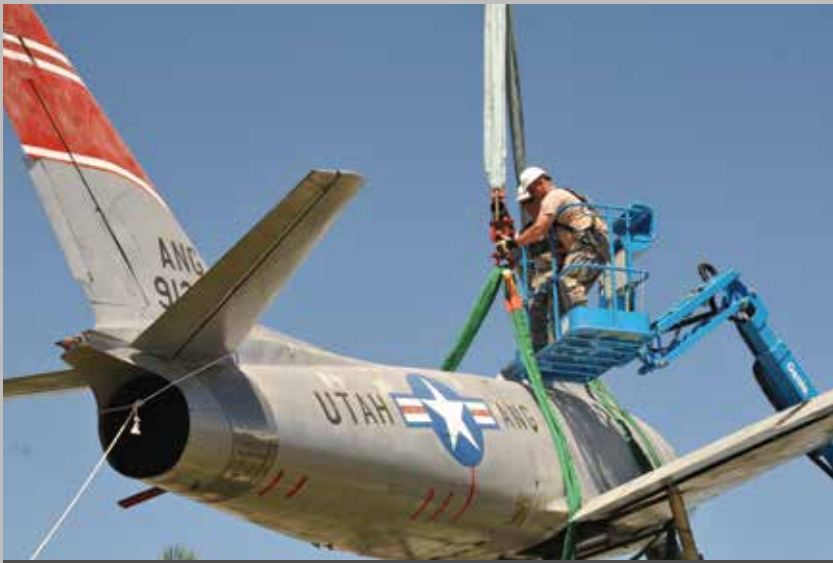
Master Sgt. Darrel Chadwick and Tech. Sgt. Fredrick Smith attach support equipment to unmount the Utah Air National Guard's F-86 that has been in front of the Draper Headquarters building for many years. Plans are to restore the F-86.
